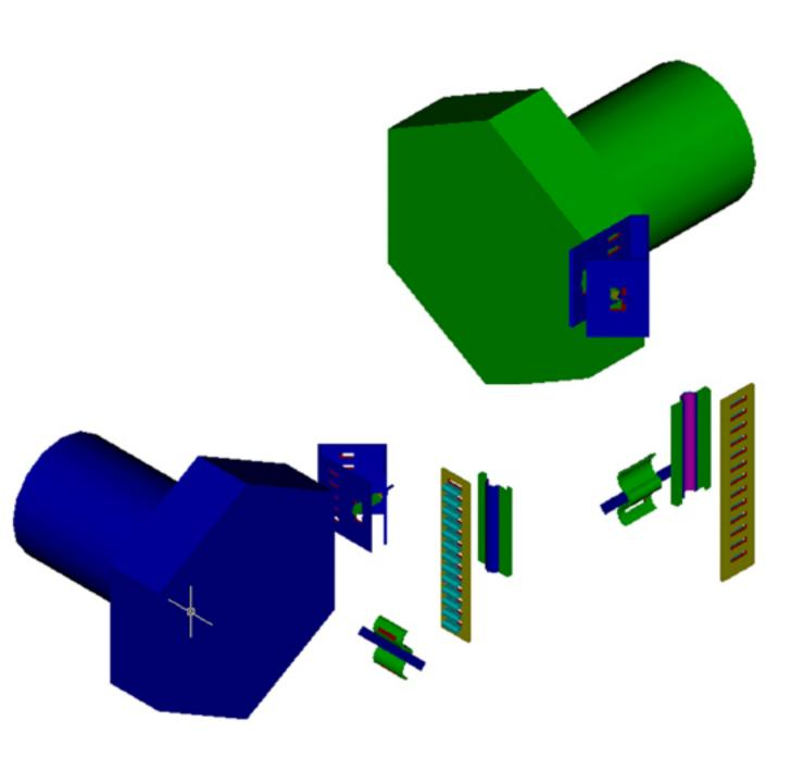
This is all the parts. The hook holders and pressure points are placed in key areas around the bolt. They are then locked into the belt. The hooks are placed in the hook holders. Once adjusted the cable tie which is placed inbetween the belt and flexable tube. Once everything is in place the cable tie is tightened and the parts are secured around the bolt. Once everything is in place it is time to turn the hooks and loosen the bolt.
